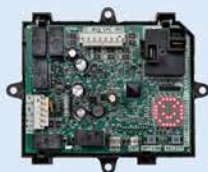
Heat Pump Defrost Control
