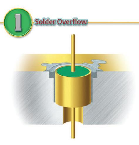
**Problem:** Solder overflow is the appearance of uneven solder flowing out of and around the solder joint area. In addition to being a visual reason for part rejection, overflowing solder is cause for concern.
