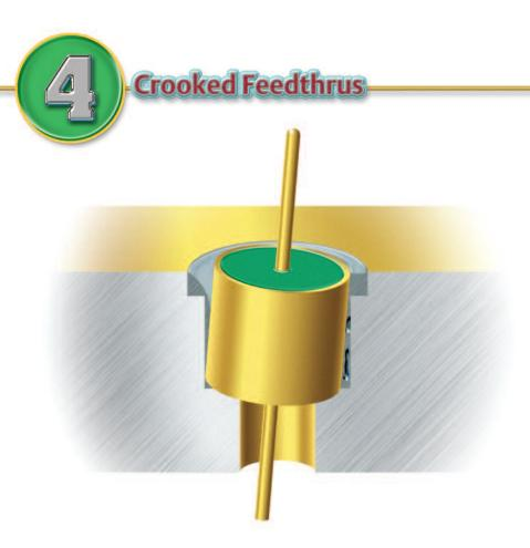
**Problem:** When the body of a feedthru is not flush with the housing this is a visual clue that the body shell is not parallel with the walls of the hole. A crooked feedthru is also an indication of an uneven soldered joint and therefore a weak point and reason for failure upon inspection.
