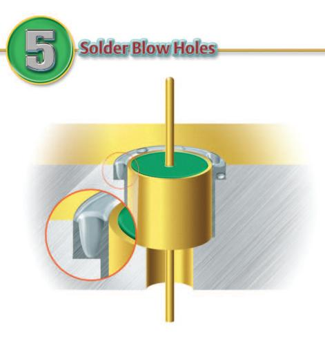
**Problem:** Voids in a solder joint will visually appear as pin holes or have a crater like or "blow hole" appearance where the bottom of the void is not visible. Both of these appearances are reasons for rejection and concern for the integrity of a solder joint.
