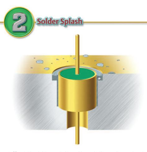
**Problem:** Solder splash is recognized by small bursts of solder extending away from the solder joint.
