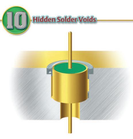
**Problem:** The most difficult, and perhaps the most dangerous pitfall of all, is when voids are out of sight. Hidden voids can be a cause for mechanical failure or hermeticity loss over time. Electrical performance may also be in jeopardy.
