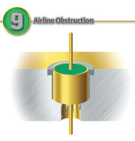
**Problem:** Airline obstructions caused by uncontrolled solder flow creates an improper ratio of pin diameter to aperture diameter which determine the ohmic impedance value.
