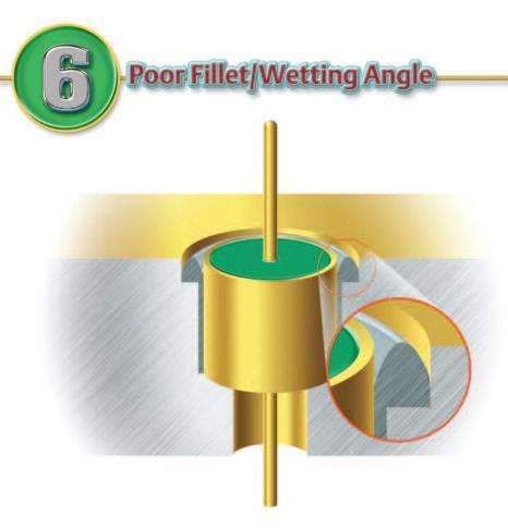
**Problem:** A poor wetting angle, or lack of wetting, is an indication that there is improper solder flow and thus poor bonding. A good solder joint will have an angular fillet at the base of the joint, a strong wetting angle is an indication that the solder joint has a strong bond.
