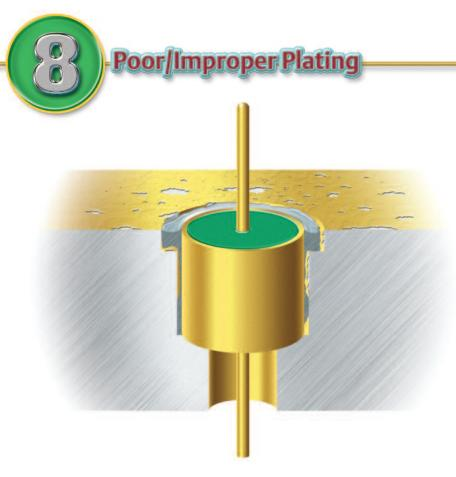
**Problem:** Blisters, voids or flaking of the plating in the solder joint area can lead to poor solder adhesion and therefore a weak joint that may later result in a hermetic or electrical failure. While the plating finish may be correct for the base metal, the plating selection also needs to match requirements for adherence to the filler metal used in the solder joint.
