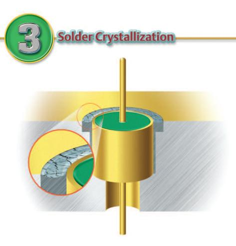
**Problem:** Solder crystallization is characterized by a cracked and uneven appearance of the solder joint. Although not necessarily an immediate cause for visual rejection, crystallization in the joint may indicate a poor solder joint that will fail over time and should be corrected.
