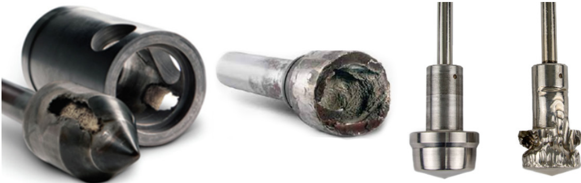
Figure 1. Erosion of valve components due to very high pressure drop
