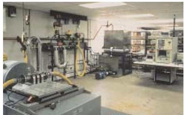
Flowing shaker table: note NIST traceable gravimetric weigh tank
