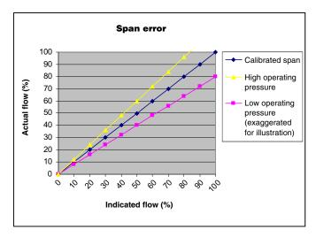
In some flowmeters that use Coriolis technology, pressure can cause a span error. Span is a generic term describing a coefficient used to establish a device's linear relationship between its input and output over a given operating range. The size and design of the meter determines whether it will have an effect, and by how much.
