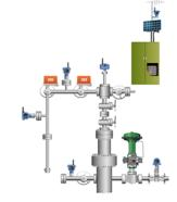
Gas Lift for Oil - controls and optimizes lift gas applied to oil-producing wells to maximize production.
