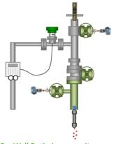
Gas Well Optimizer - monitors, controls, and optimizes your production wells. Includes deliquidification techniques such as intermitting, plunger lift, gas lift, and more.
