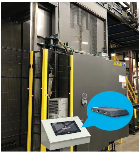
The Emerson RXi2-LP industrial PC brings all sensor data together for accessibility, historian, visualization, and analysis for primary product packaging machines or complete packaging lines. In addition, real time monitoring and diagnostics capabilities enable better OEE.
