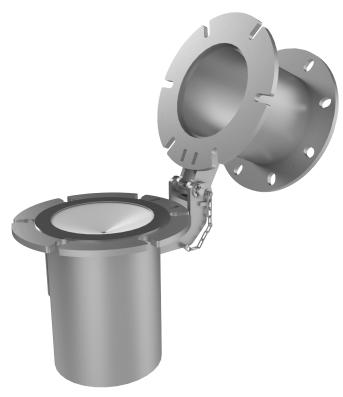
Rosemount TGS 68 Tank Gauge Socket, Hinged Heat Protection, is a socket for mounting the Rosemount TGU 68 Tank Radar Gauge when used on heated cargoes such as Bitumen. The hinged socket with the removable separation disc makes it easy to clean the antenna and separation disc. The TGS 68 makes it possible to use the TGU 68 with cargo tank temperature up to 260 degrees Celsius.
