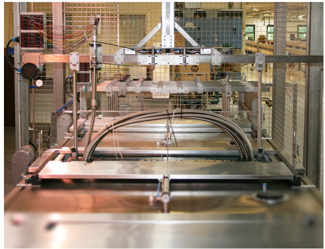
Figure 1. Calibration Station for Accurate State-of-the-Art Sensor Elements
