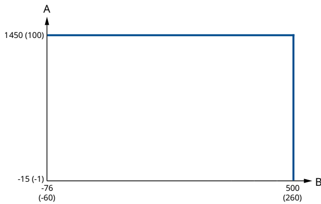
Figure 14: MTMP - Medium Temperature and Medium Pressure (Code M)
