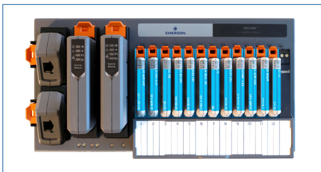
IS CHARM I/O Block with redundant Scanner Modules and IOPs, a combination of IS CHARMS and Channel Identifier Label/Wiring Cover.
