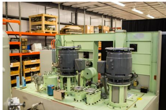
Figure 2. Interior view of a large Pelton cabinet actuator
