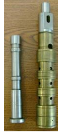
Figure 4. Pilot valve cage and spool
