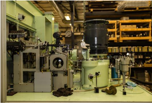
Figure 3. Pelton flyball assembly, distributing valve
