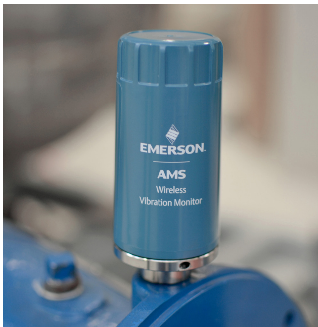
Figure 2. Wireless vibration monitor.
