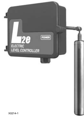
Figure 2-16. In the upstream oil and gas industry displacer type liquid level controllers along with on/off dump valves are used for controlling liquid level in oil and gas production separators. The controllers use a displacer sensor to detect liquid level or the interface of two liquids of different specific gravities. The output signal from the controller is either electric or pneumatic and sent to an on/off dump valve to open or close it. The L2e shown is the electric output version of this controller.
