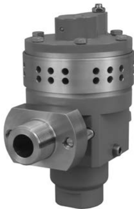
Figure 2-14. On fast control loops, a positioner may not be able to react quickly enough to be of use. In these situations, performance of spring-and-diaphragm actuators can be improved by use of pneumatic boosters such as the SS-263.
