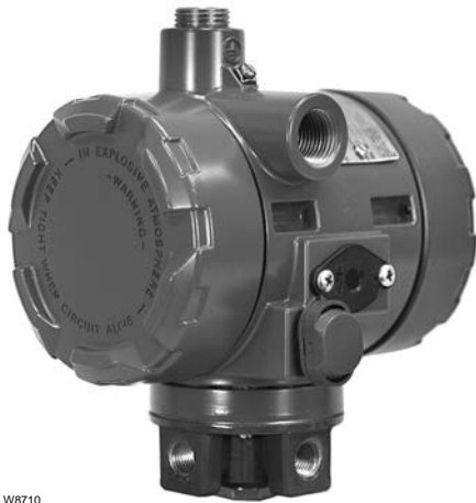
Figure 2-13. Electro-pneumatic transducers are a common actuator accessory. They take a milliamp signal and produce a proportional pneumatic output. The i2P-100 is compact, accurate and has low air consumption.
