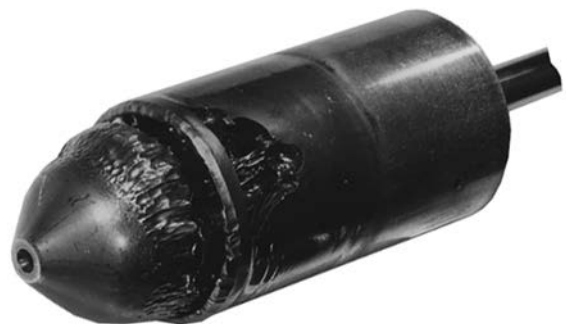
Figure 6-6. The top plug shows the characteristic rough texture of cavitation damage, which differs greatly from the polished appearance of damage due to flashing (lower photo). The two damage mechanisms vary greatly.
