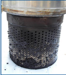
Harsh environments paired with poor maintenance procedures can lead to valve damage, like the plugged cage pictured above.
