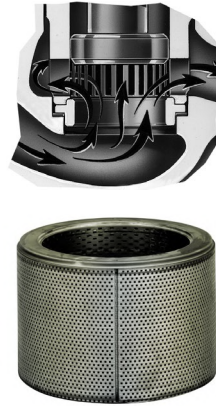
Figure 5.10 Valve Trim Design for Reducing Aerodynamic Noise
