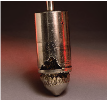
Figure 5.8 Typical Appearance of Flashing Damage
