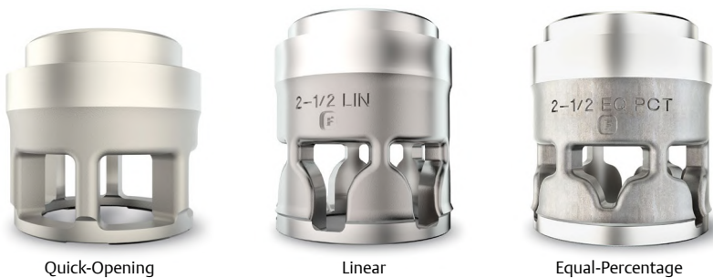
Figure 3.37 Characterized Cages for Globe-Style Valve Bodies
