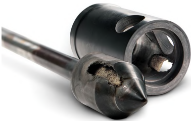
Figure 5.9 Typical Appearance of Cavitation Damage
