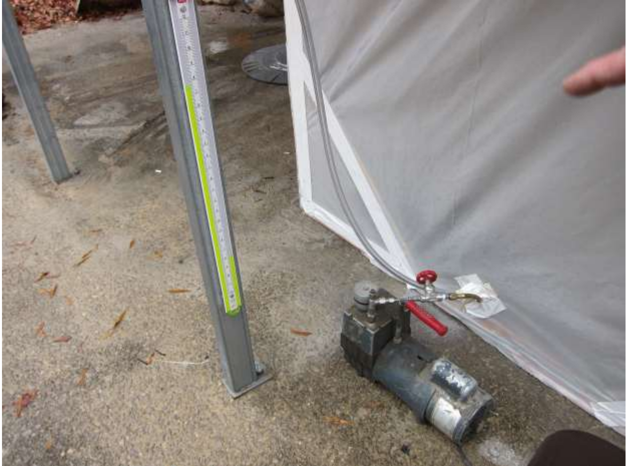
Photograph No. 2 Protection Against Solid Foreign Objects (Dust-Tight) Test Setup
