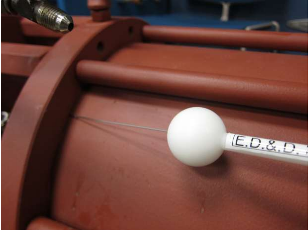
Photograph No. 10 Protection Against Hazardous Parts Test Setup
