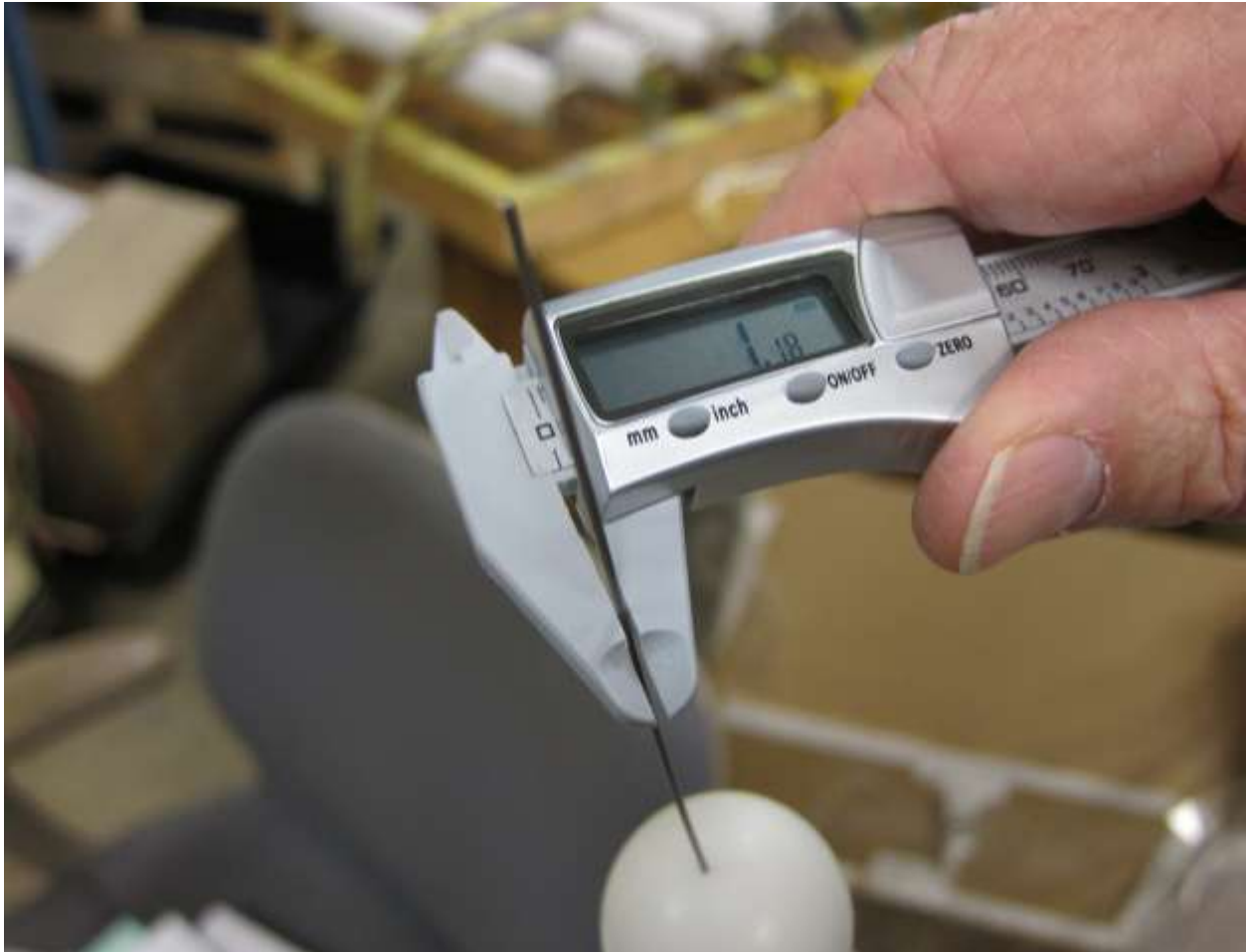
Photograph No. 12 Protection Against Hazardous Parts Test Setup
