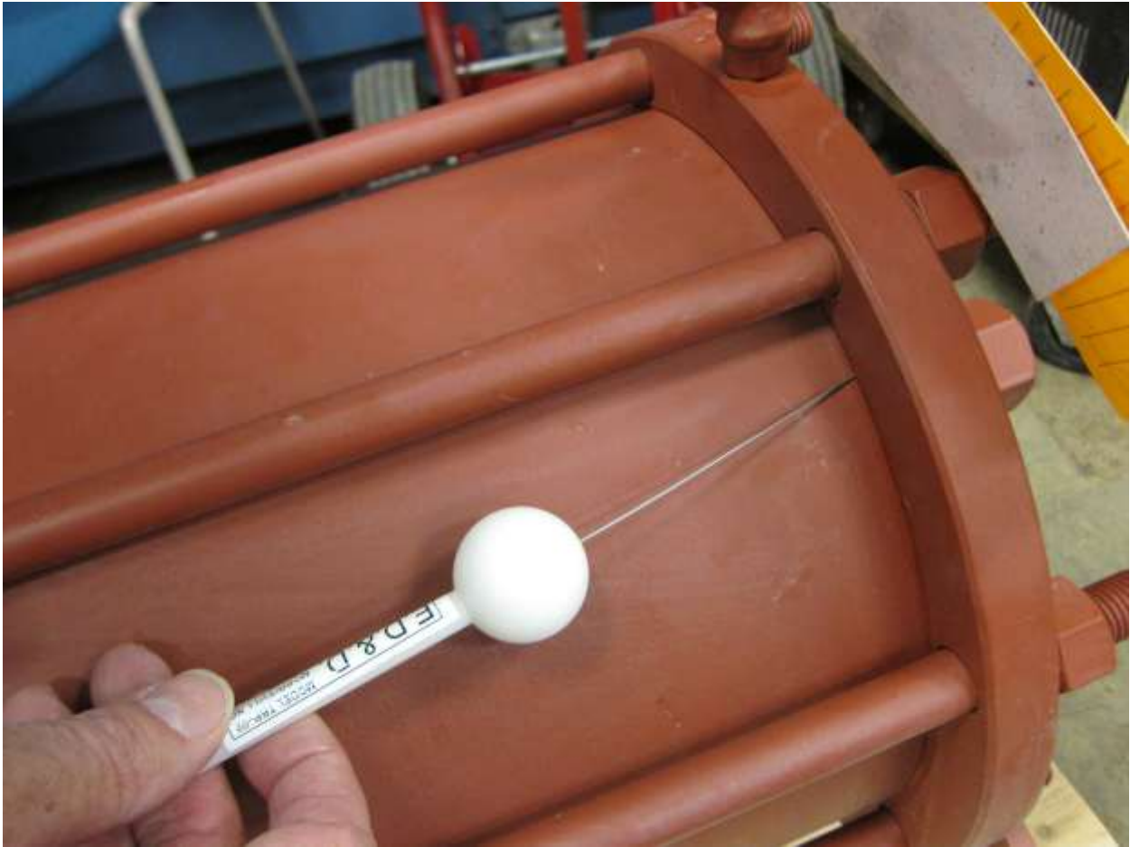
Photograph No. 9 Protection Against Hazardous Parts Test Setup
