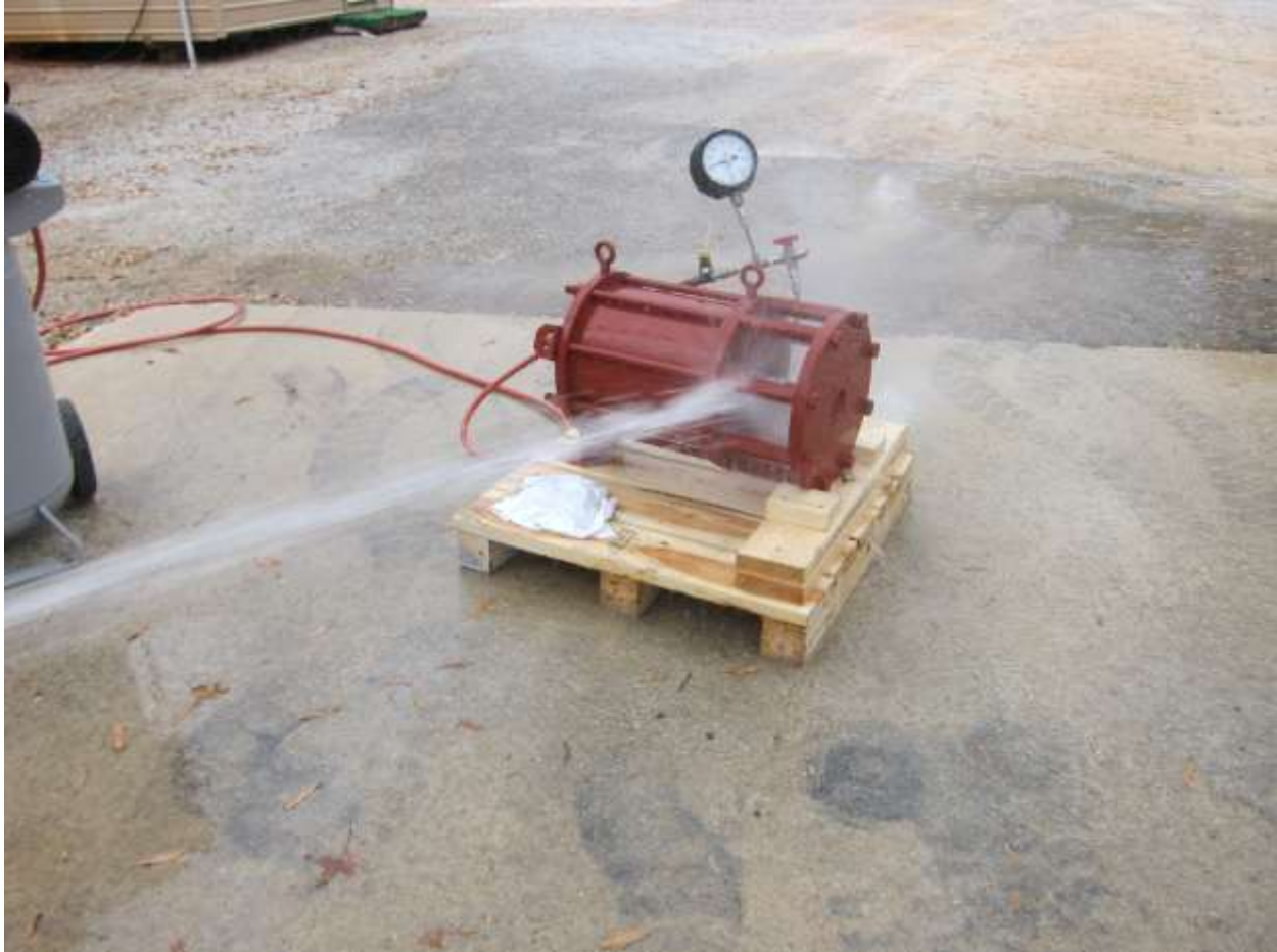
Photograph No. 8 Protection Against Ingress of Water (IP66M) Test Setup
