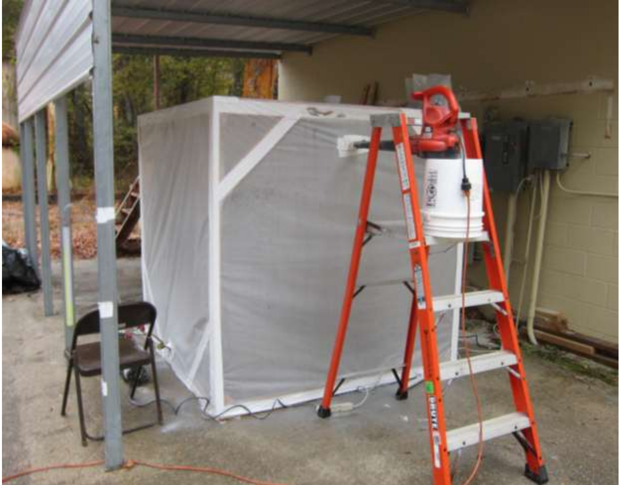
Photograph No. 1 Protection Against Solid Foreign Objects (Dust-Tight) Test Setup
