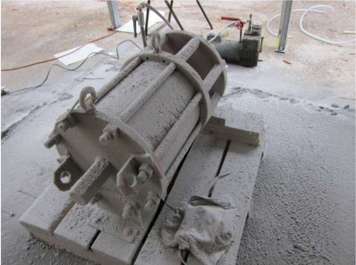
Photograph No. 4 Protection Against Solid Foreign Objects (Dust-Tight) Test Setup (Post-Test Appearance)
