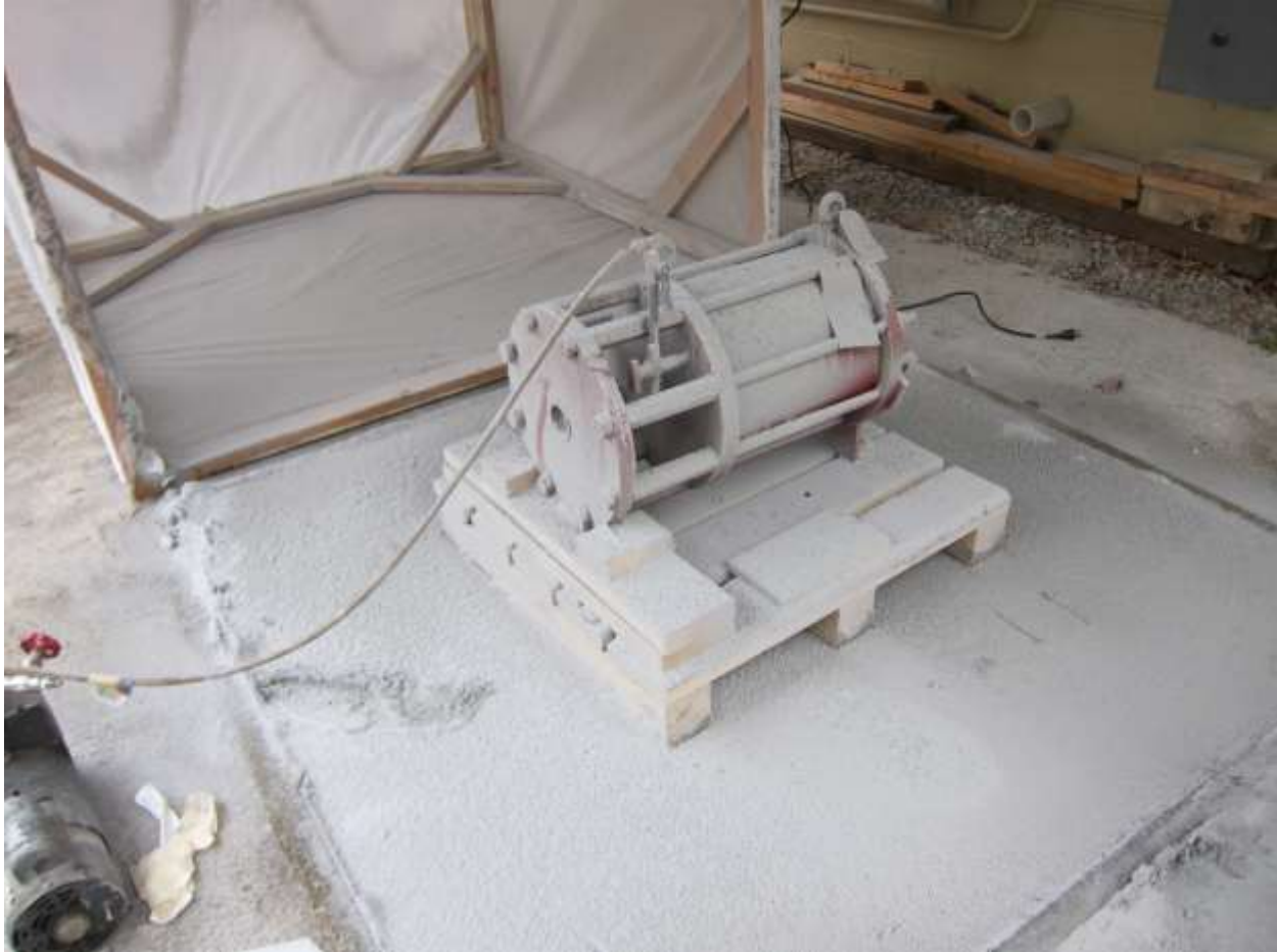
Photograph No. 3 Protection Against Solid Foreign Objects (Dust-Tight) Test Setup (Post-Test Appearance)
