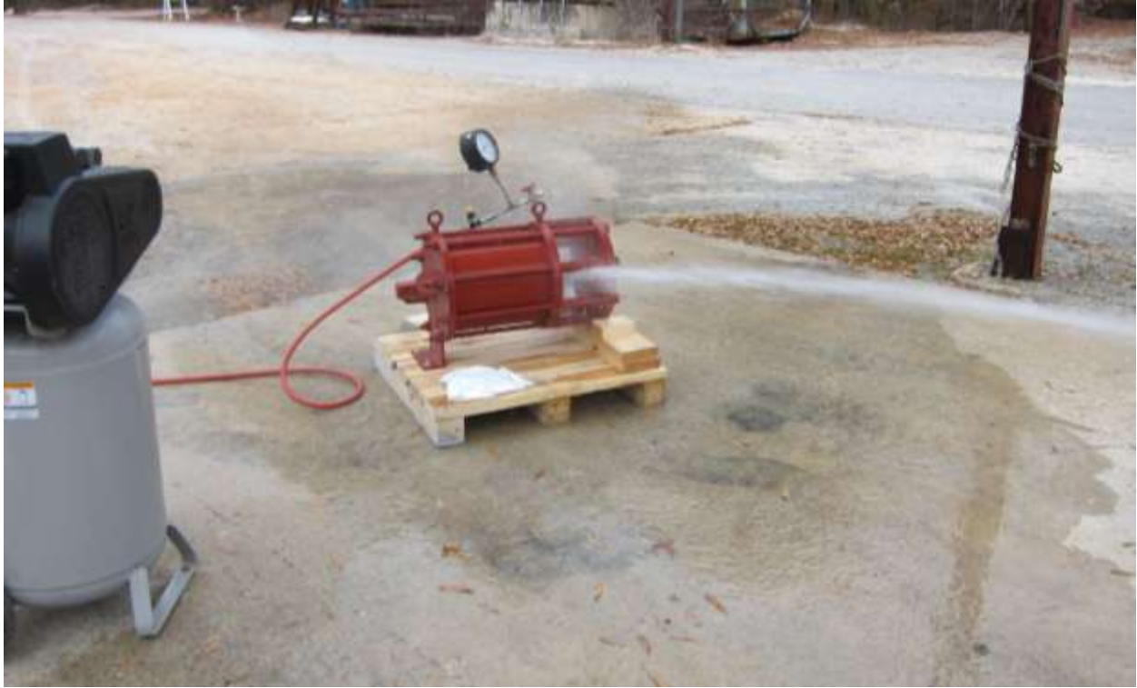
Photograph No. 7 Protection Against Ingress of Water (IP66M) Test Setup
