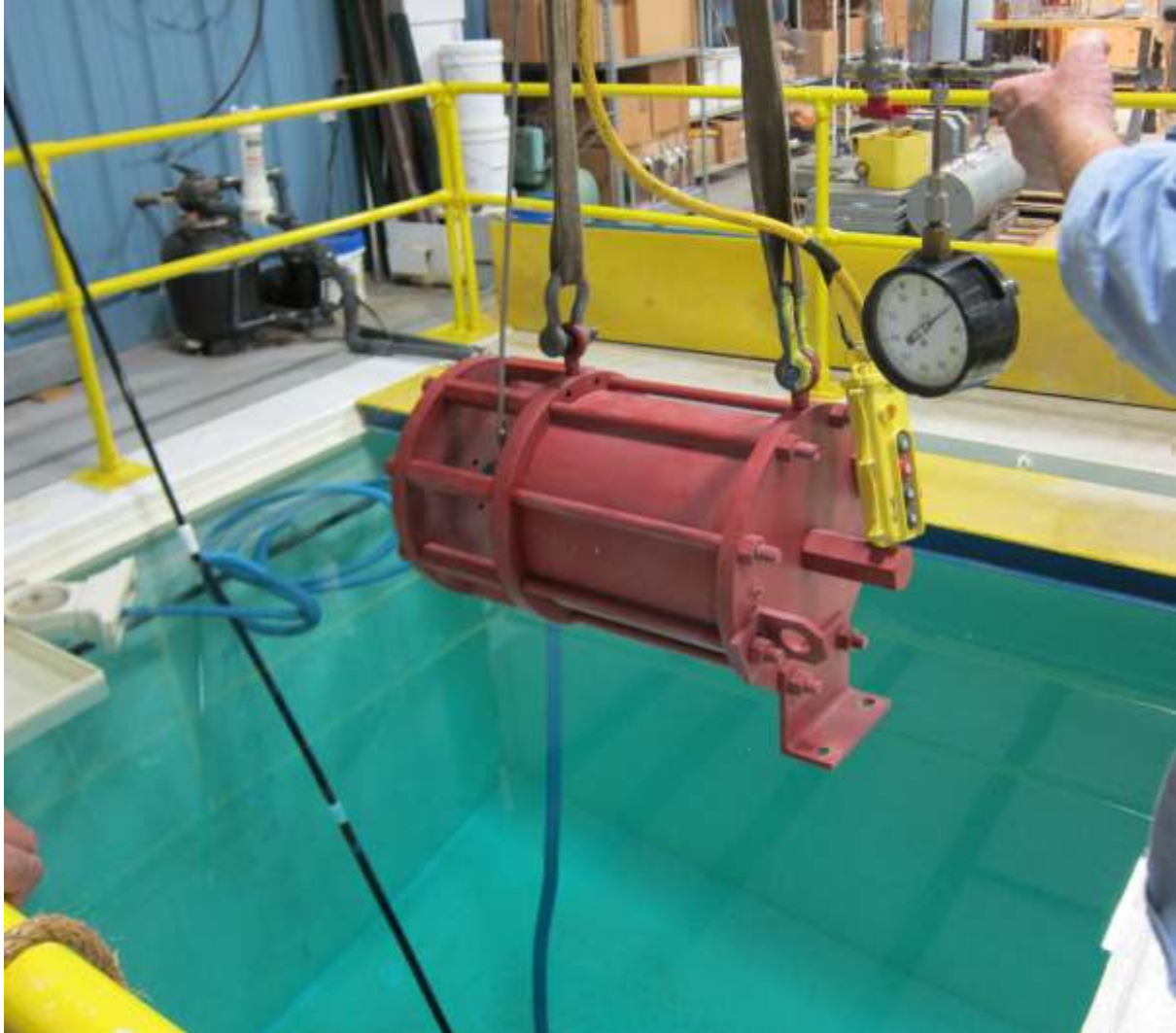
Photograph No. 5 Protection Against Ingress of Water (IP67M) Test Setup
