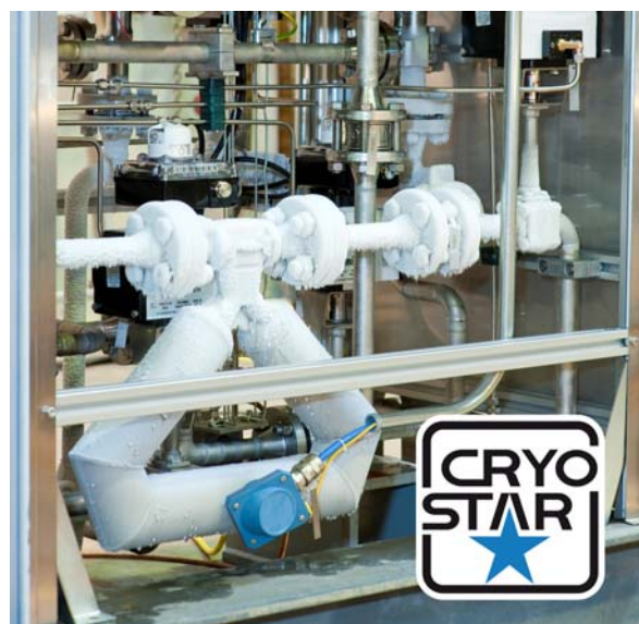
Cryostar LNG dispenser with Micro Motion ELITE Coriolis meter
