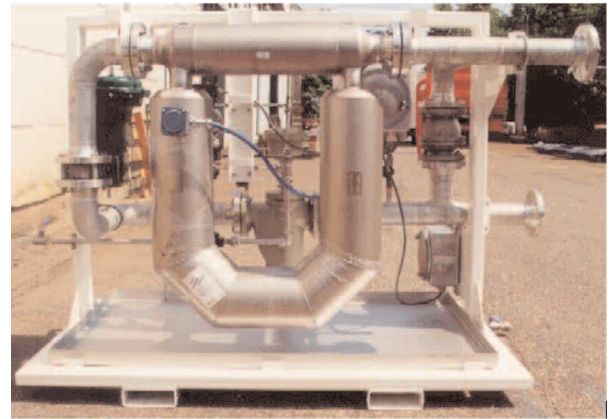
Mobile metering skid with Micro Motion sensor.
