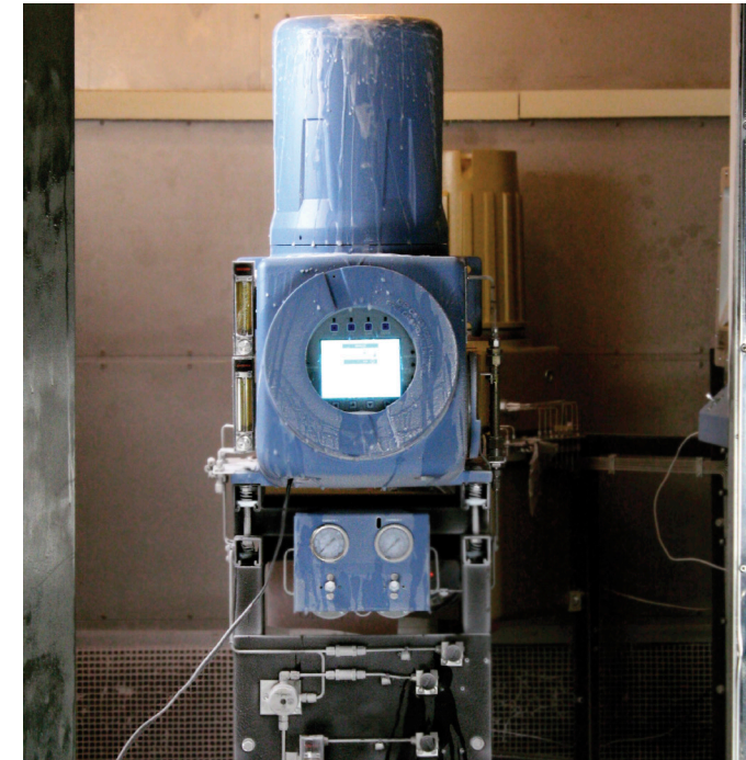
Rosemount 770XA gas chromatograph shown inside the environmental testing chamber.
