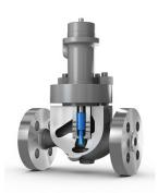
Cage, plug, and seat ring are designed and manufactured as a unit, offering cavitation control for high pressure drops at very low flow rates
