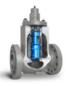
Uses a series of large area flow restrictions and expansions to control the pressure drop of the fluid while allowing particulate to pass
