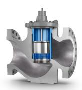
Up to 18 dBA noise reduction - Designed with small vertical slots around the circumference of the cage to reduce turbulence within the flow passages
