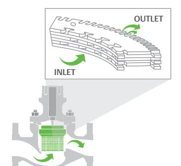
Unique Flow Passage Shapes reduce turbulence to minimize shockassociated noise and place turbulent shear layers away from solid boundaries to reduce noise. The multi-stage pressure reduction, utilized with sound engineering principles, controls jet size, formation, interaction, and accommodates fluid expansion.
