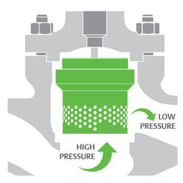
Pressure Management utilizes the expanding area principle to allow for volumetric expansion of depressurizing gas and safe pressure reduction of potentially cavitation liquids.
