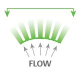
Exit Jet Independence is crucial for avoiding jet coalescence, which will lead to additional noise. All Emerson noise technologies are designed with this critical factor as standard.
