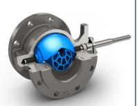
Features an attenuator welded on the back of the V-notch ball, which separates the flow into multiple smaller jets
