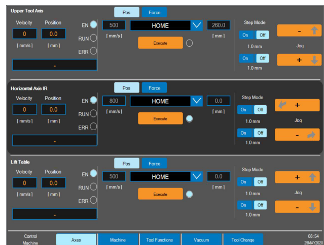
Parameters for lower servo driven lift table.
