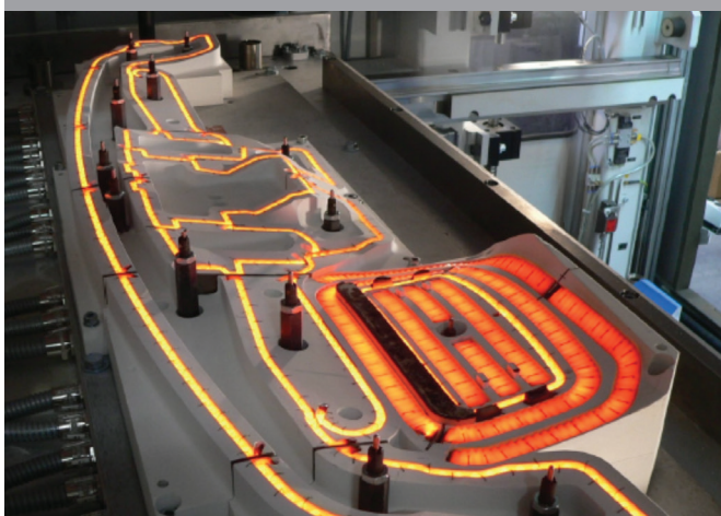
CIT allows for clean joining of large, contoured parts such as the housing for instrument cluster and the HVAC ductwork behind a dashboard.
