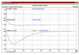
Users may test the solution in a simulator that shows the loop reaction to set point changes, load disturbances, and cyclic variation. Simulation results can be displayed in either frequency domain (Bode plot) or as time response. The user learns what variability can and cannot be removed and what limitations are imposed by the process.
