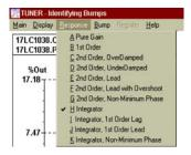
Intuitive drop down menus allow the user to select the type of dynamic response that the control loop best represents. Control loop tuning - no longer "tune-by-feel". Backed by Emerson's training and support services, the user will implement realistic and mathematically sound control tuning changes, based on understanding of process dynamics, the analysis and recommendations provided by the Toolkit, and effective tuning strategies.
