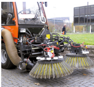
◀ Cylinder valve unit for positioning and adjusting brushes
