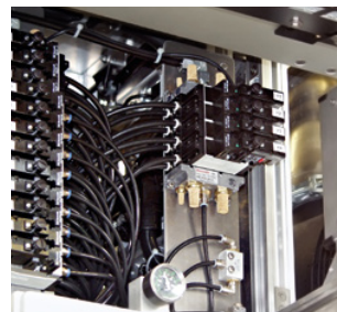
▲ Valve systems with maintenance unit, complex control with CANopen bus technology - Valve system, CD01 series - Maintenance units, NL2 series
