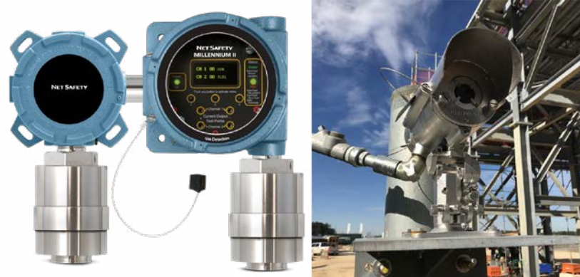
Figure 16: Fixed point combustibles and toxic gas detectors use multiple sensor technologies, such as infrared, catalytic bead and electrochemical. The Net Safety Millennium II series (left) can detect all flammable gases and common toxic gases. Rosemount 935/936 Open Path Combustible and Toxic Gas Detectors (right) use infrared and ultraviolet technology to detect hydrocarbon and toxic gases, including methane, propane, ethylene, hydrogen sulfide and ammonia.
