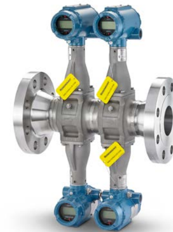
Figure 3: Flow meters, such as the Rosemount™ 8800 Quad Vortex Flow Meter, provide the ultimate redundant flow measurement solution to guard against spurious trips using 2oo3 voting, plus a fourth integrated transmitter for process control.
