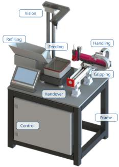
The aflex compact system is a standardized pick and place system for efficiently providing small parts in any desired position. The solution features:
