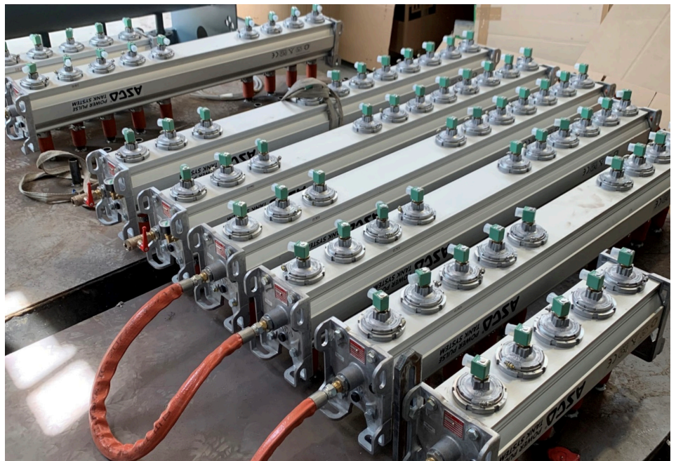
An example of a solution provided by Emerson to equip an 8-MW (27 MMBtu) biomass boiler. It consists of ASCO Series 355 tanks with immersed ASCO Series 353 valves.
