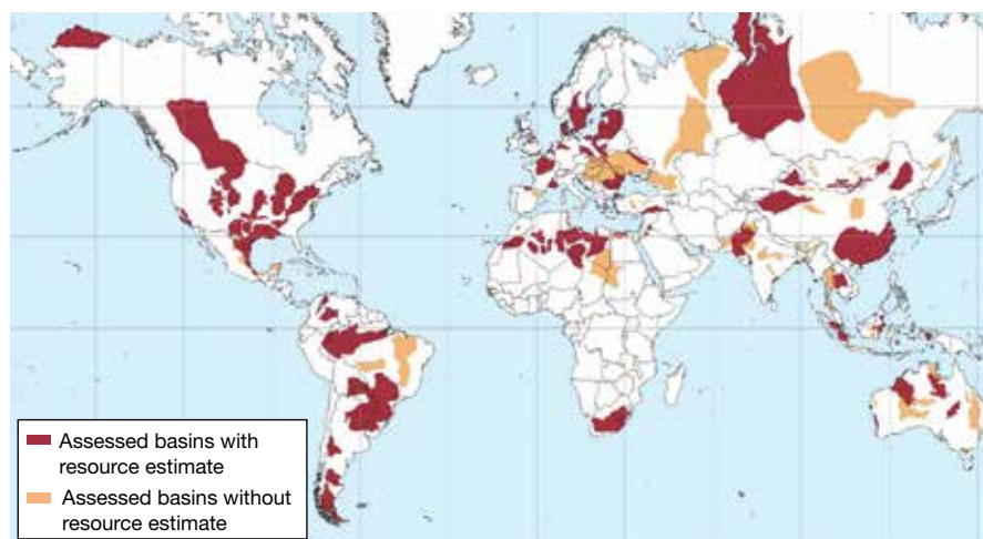
◀ Figure 1. Tight oil is found throughout the world, as shown in this map of basins with shale oil and shale gas formations. The red areas represent basins with shale formations for which the U.S. Energy Information Administration (EIA) estimated recoverable oil and natural gas resources; the tan areas represent basins that were reviewed, but for which the EIA did not provide shale resource estimates, mainly due to the lack of data necessary to conduct the assessment. Source: (1).
