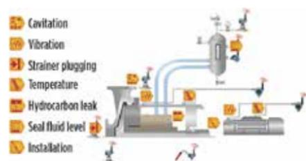
FIG. 1. A refinery pumping system with wireless transmitters.
