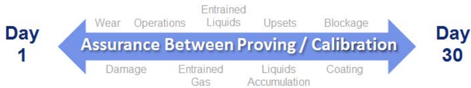
Figure 5. Diagnostics can be used to detect many upset conditions between proving cycles
