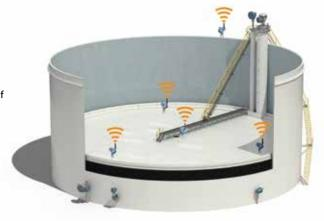
"Both the Rosemount 3308 and the Rosemount 5900C are radar level gauges using similar principles, where the 5900C is the premium choice for floating roof monitoring, whilst the 3308 has the advantage of being fully wireless," says Hoffmann.
