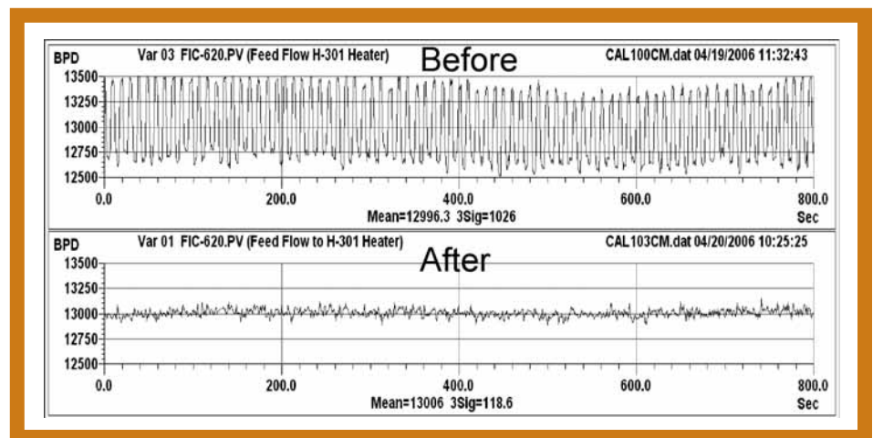
Figure 6: A high-performance digital positioner provides an 88% reduction in process variability.
