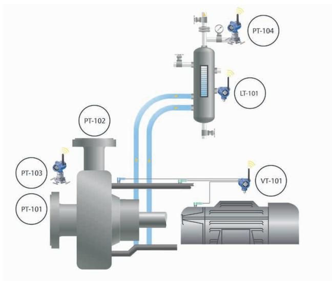
**Figure 2. Pump monitoring diagram.** A wide variety of parameters are typically measured on pumps used in pipelines, some of which are depicted in this diagram.
