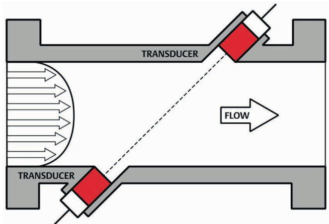
Figure 3. Ultrasonic instruments transmit and receive pulses diagonally across pipes to measure fluid flow.
