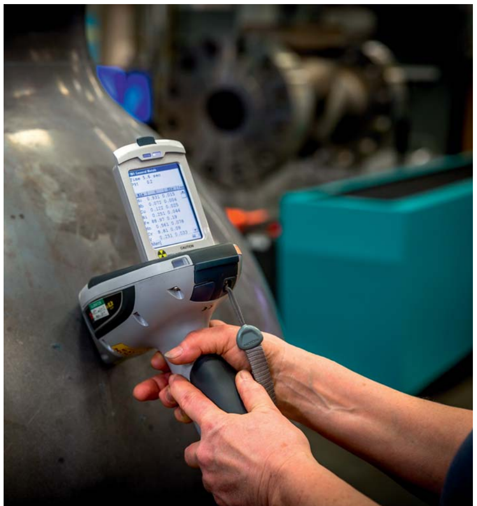
Figure 2: A PMI gun can identify the alloy being used in a valve part. Here, it is analyzing the valve body of a Fisher™ valve.
