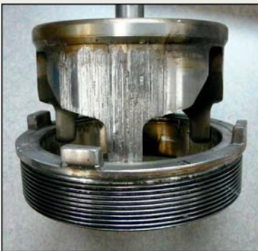
Failure to harden trim components as intended by the OEM could result in galling of metallic surfaces, such as the trim and plug shown.
